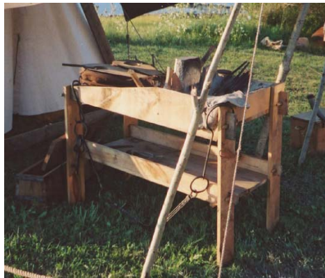
The Viking all wood forge and its double bellows used to blow the flame.
