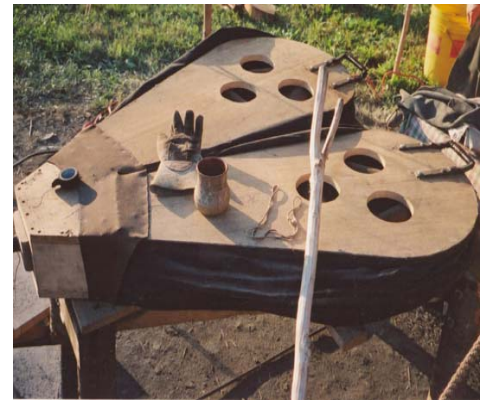
The Viking all wood forge and its double bellows used to blow the flame.
