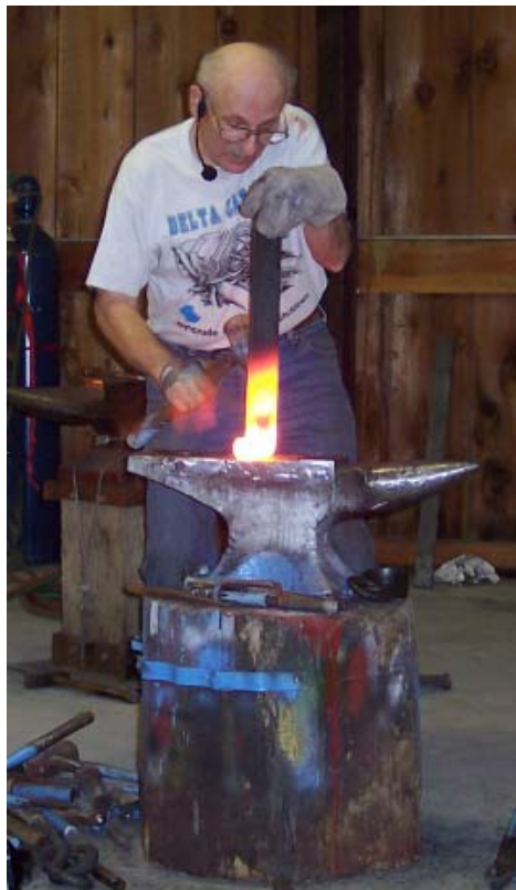
John Adolph said that a lot of the work for smiths in the past had been the making of springs for automobiles. He demonstrated the forging of the part where the spring is bolted to the frame of the car.
