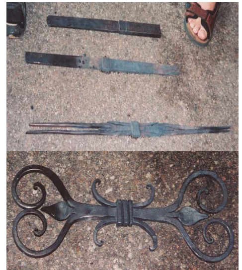
Evolution of a filler panel done by Fred Crist. Top to bottom: 1. original stock, 2. partially forged to shape, 3. cut and ready to form, 4. the finished piece. All one piece but looks like it was made from several pieces.
