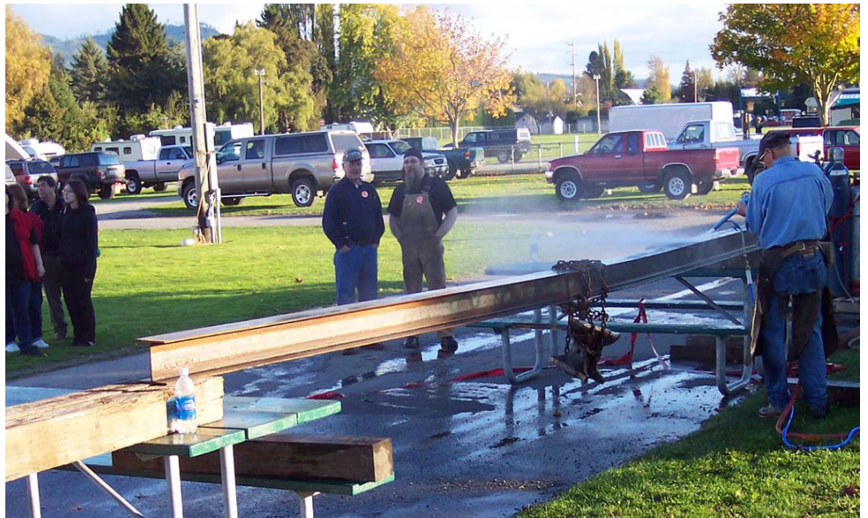
John Adolph demonstrating beam bending by heating and cooling.
